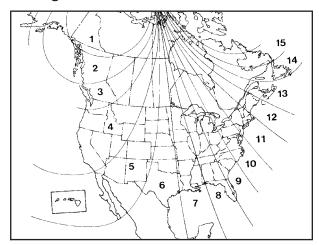
Turn the ignition on and cycle the DIC to the Compass/Temperature mode. Press the RESET button for about five seconds. The last entered variance
